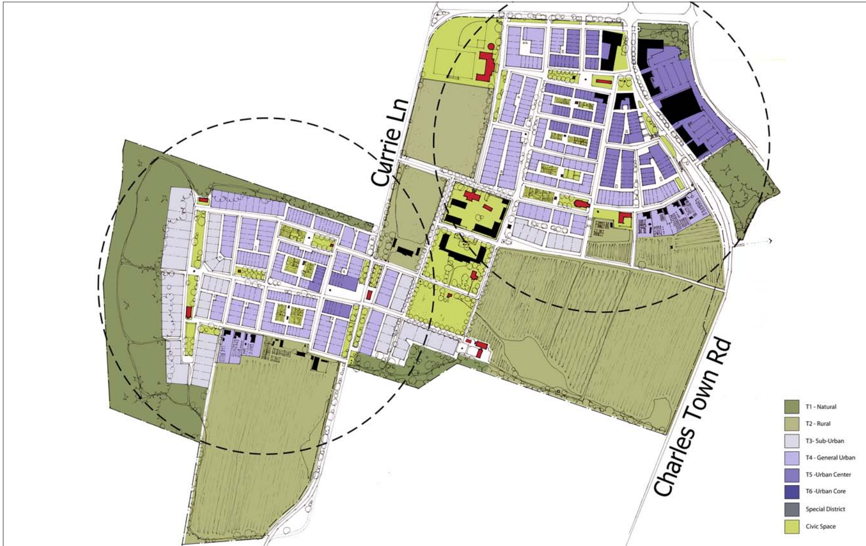
Regulating Plan of one Transect-based zoning option. This achieves entitlements similar to those possible under the old TND ordinance.
