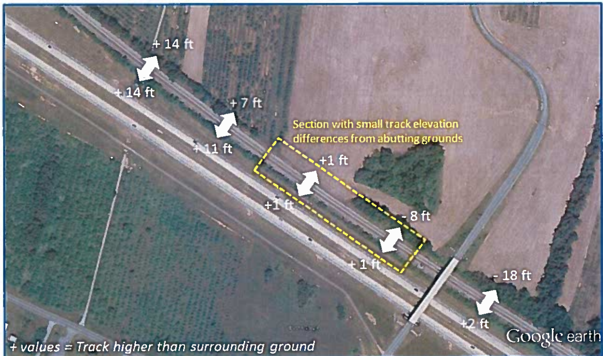
Figure 9 – Track Elevation Differences at Jefferson Orchards
