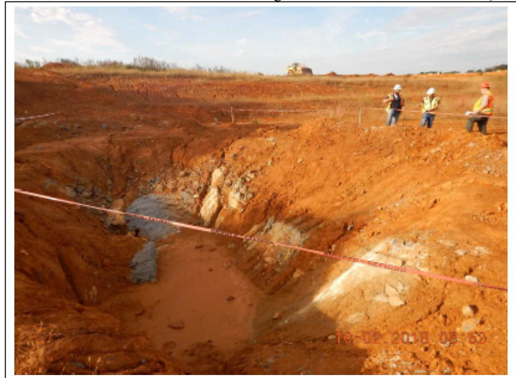
Figure 6. Closed depression or sinkhole in the Central Folded Carbonate Unit hydrogeologic area of northern Jefferson County (WVDEP 2018) in the general vicinity of the northern end of the Route 9 Sewer Project. All of the rock and soil where the depression is now has moved down through fractures into solutionally-enlarged voids in the bedrock beneath. This sediment is, in turn, a contaminant in groundwater (photographer not named).
