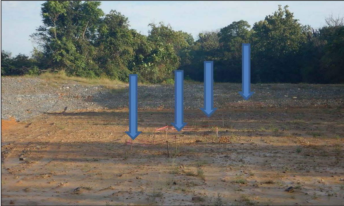
Figure 8. Four sinkholes in the RAN 5 Project Reuse Pond. (WVDEP 2018a) (photographer not named).
