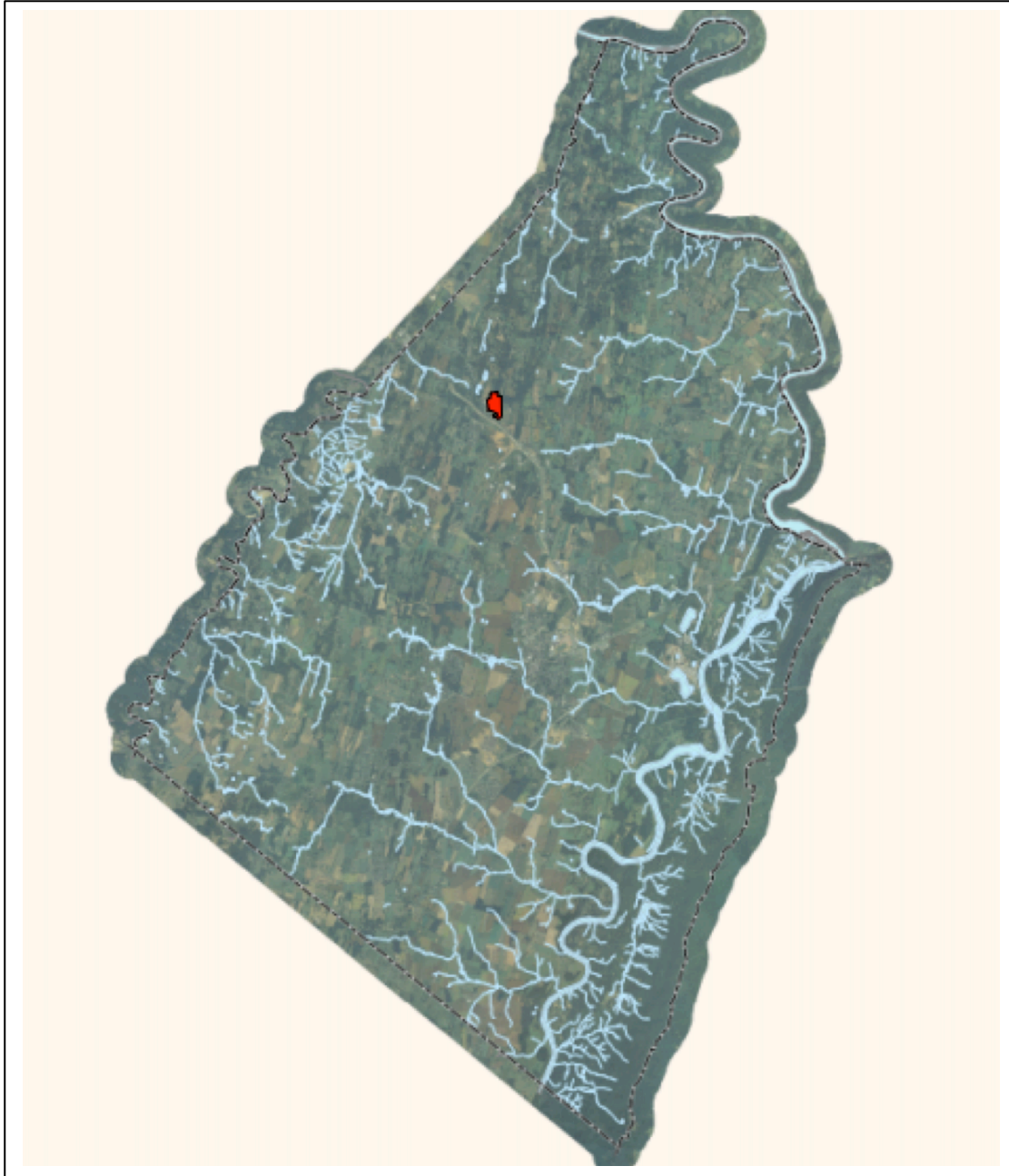
Figure 7. Surface drainage (light blue lines) in Jefferson County. It can be clearly seen that surface flow in the part of the county in the vicinity of the RAN Project is almost wholly lacking. This map has been modified (approximate facility added) from Meloy and Carter (2012).
